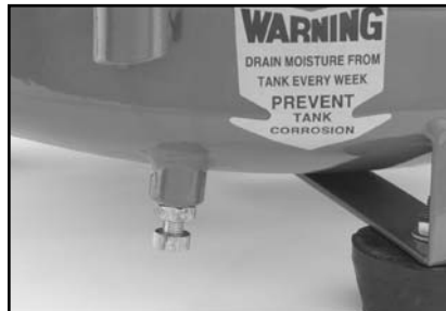
Figure 5. Drain valve location.
